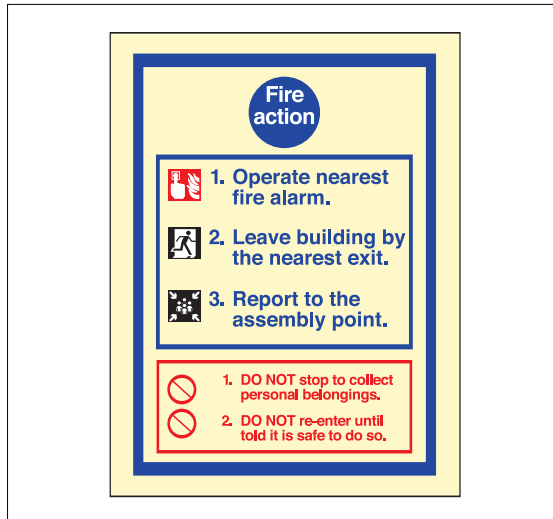
Figure 11: Simple fire action notice
