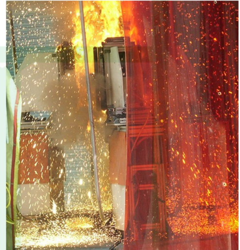
Figure Electrical arc blast
