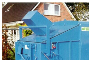
f. Waste Compactor
