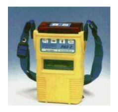
For construction work most atmospheric testers are set up to detect for deficiency of oxygen, methane gas and hydrogen sulphide. Most atmospheric monitors have the facility to attach other sensors.
